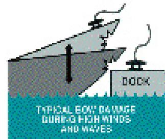
If mooring to pilings, place a 2" x 12" x suitable length "fender board" between your fenders and the pilings, to protect your hull from damage.
